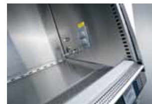
High-velocity return air slots maximize protection.
